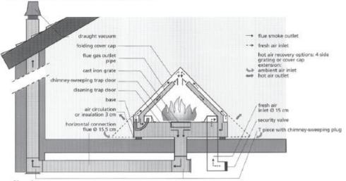
Dimensions: base sides: 1 m / with 4-side grating: 1,10 m / with cover cap extension panel: 1,30 m base height: 0,22 m / cover cap height: 0,70 m
