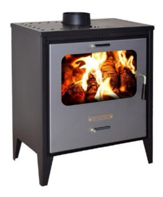
Wood Burning Stove made of 2,5 - 3,0 mm Steel equipped with tertiary combustion system (Ecoburn2), which inserts preheated air to the back side of the burning chamber and creates the conditions for secondary and tertiary combustion to take place, increasing the stove's efficiency, reducing wood consumption and lowering emissions. It also has adjustable primary and secondary air inlets. CE certifled according to EN 13240.
